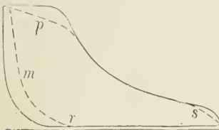
FIG. 109.— m = excess of lead; p = wiredrawing; s = early release; r = early compression.
